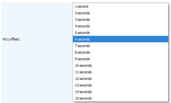
**Join accept delay 1** (not displayed in the "Simple" mode) – sets the time that the device will open the first receiving window to receive confirmation for the join request from the LoRaWAN network while OTAA mode active. The second window always opens after 1 second after the first.
