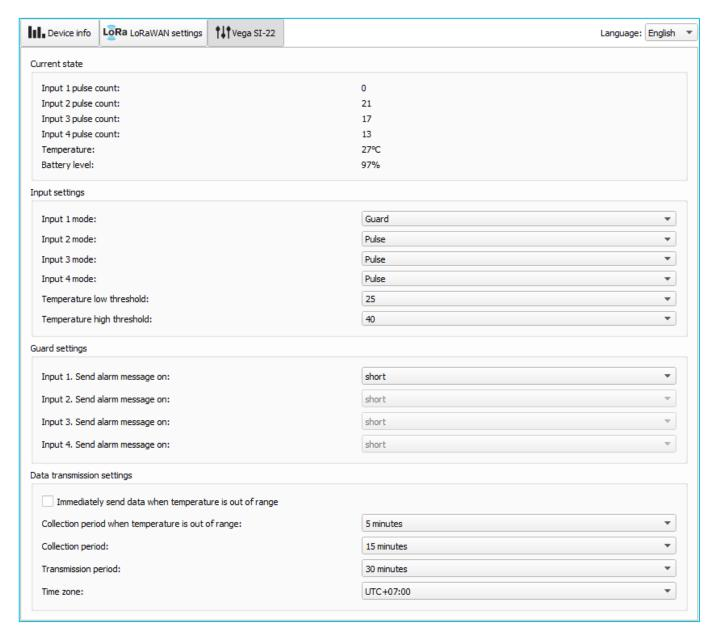
Current state – displays the current parameters of the device - the number of counted pulses at the inputs, the external thermistor temperature, and the battery level.
