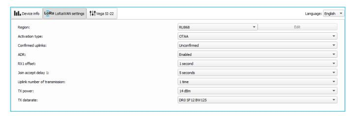
**Region** - allows you to select one of installed frequency plans or specify a custom frequency plan. Custom frequency plan is EU-868 based.
