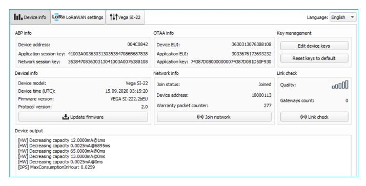
**ABP info** - displays the data necessary to register the device in the LoRaWAN network with ABP method (Activation By Personalization).
